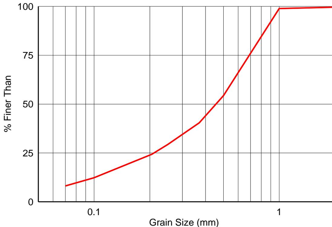
**Figure 7:** Particle size distribution of dune material (TPRC 190D) sampled from the surface 0.3 m.
