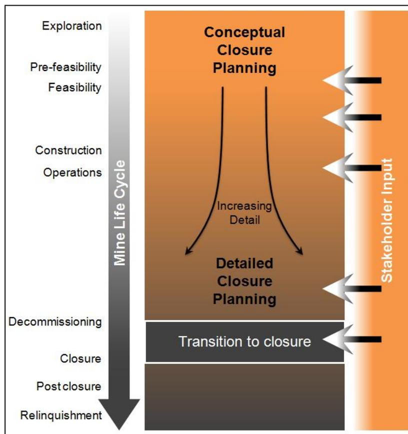
Figure 10.4: Closure planning process illustration (Adapted from International Council of Mining and Metal 2008)
