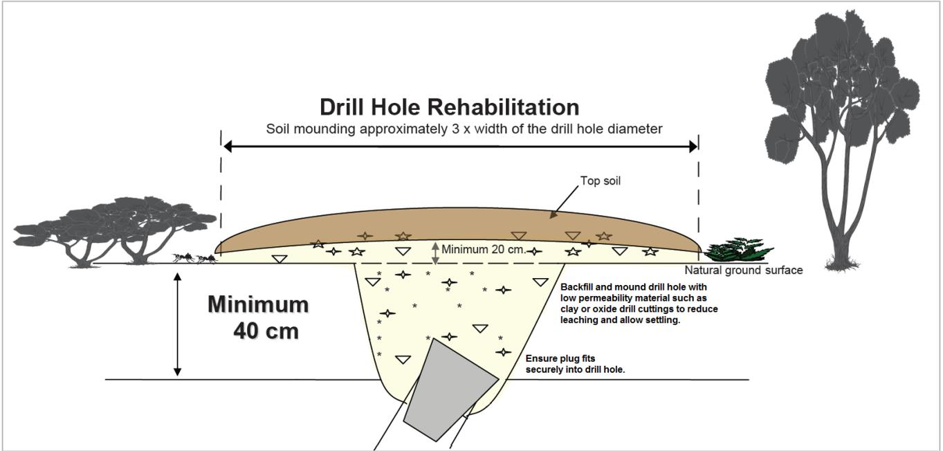
*Figure 2: AC Drill Collar Rehabilitation Spec*
