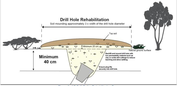
Figure 2: AC Drill Collar Rehabilitation Spec
