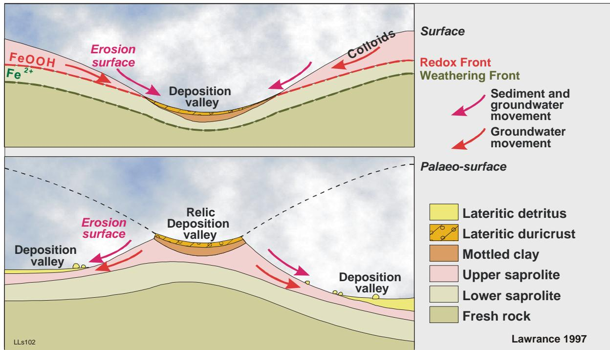
**Figure 5 Schematic representation of duricrust formation and relief inversion under wet-dry climates.**
