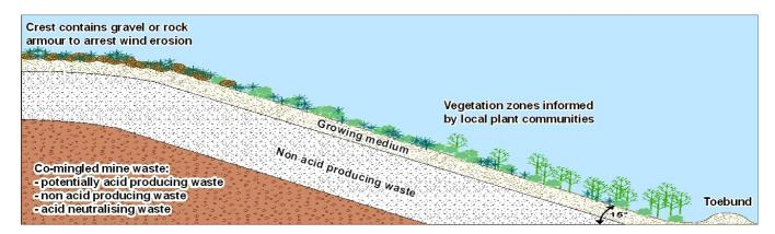
Figure 10.2: Conceptual Waste Landform Cross-section for Tropicana Gold Project
