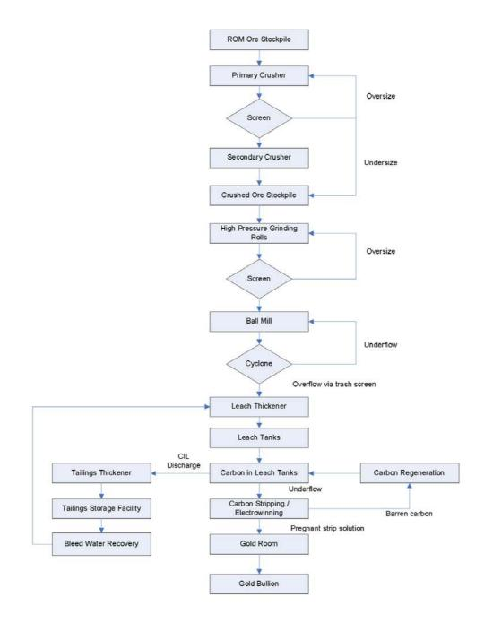
Figure 3: Processing Flow Chart - Extracted Ore to Gold Bullion.
