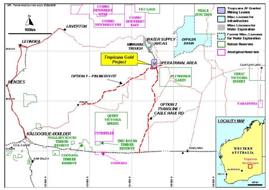
Figure 1: Tropicana Gold Project - Location of the proposed Operational Area, Mine Access Road Options and Water Supply Area Options
