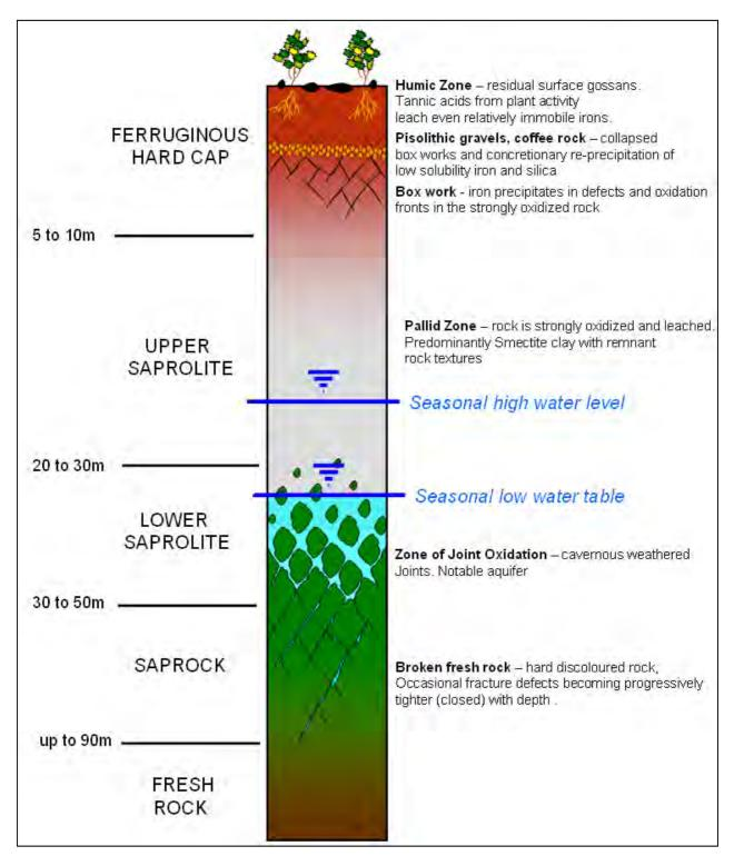
Figure 7.10: Water Table at the Operational Area and Laterite Profile (Source: Appendix 2-B17)
