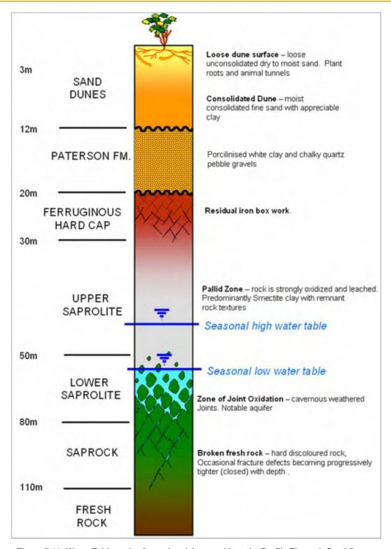
Figure 7.11: Water Table at the Operational Area and Laterite Profile Through Sand Dunes (Source: Appendix 2-B17)
