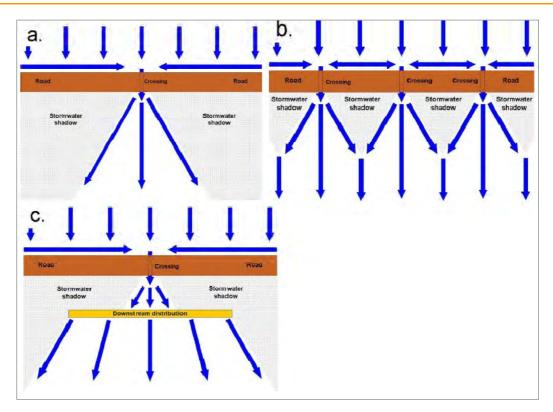
Figure 7.9: Possible Surface Water Flow Paths Downstream From a Road (Appendix 2-C3)
