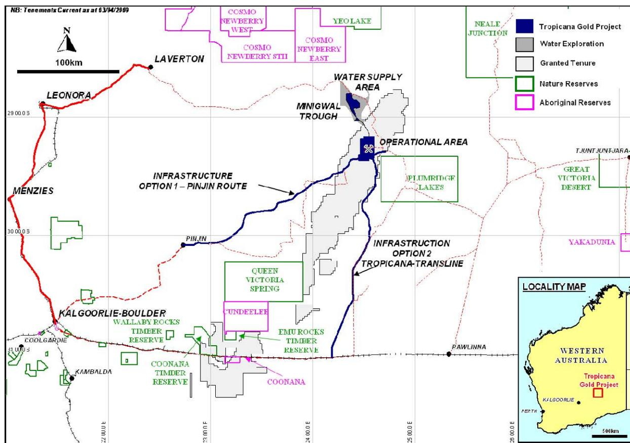
Figure 1 Layout of Proposed Mine Access Road and Infrastructure Corridor – Pinjin Option shown.
