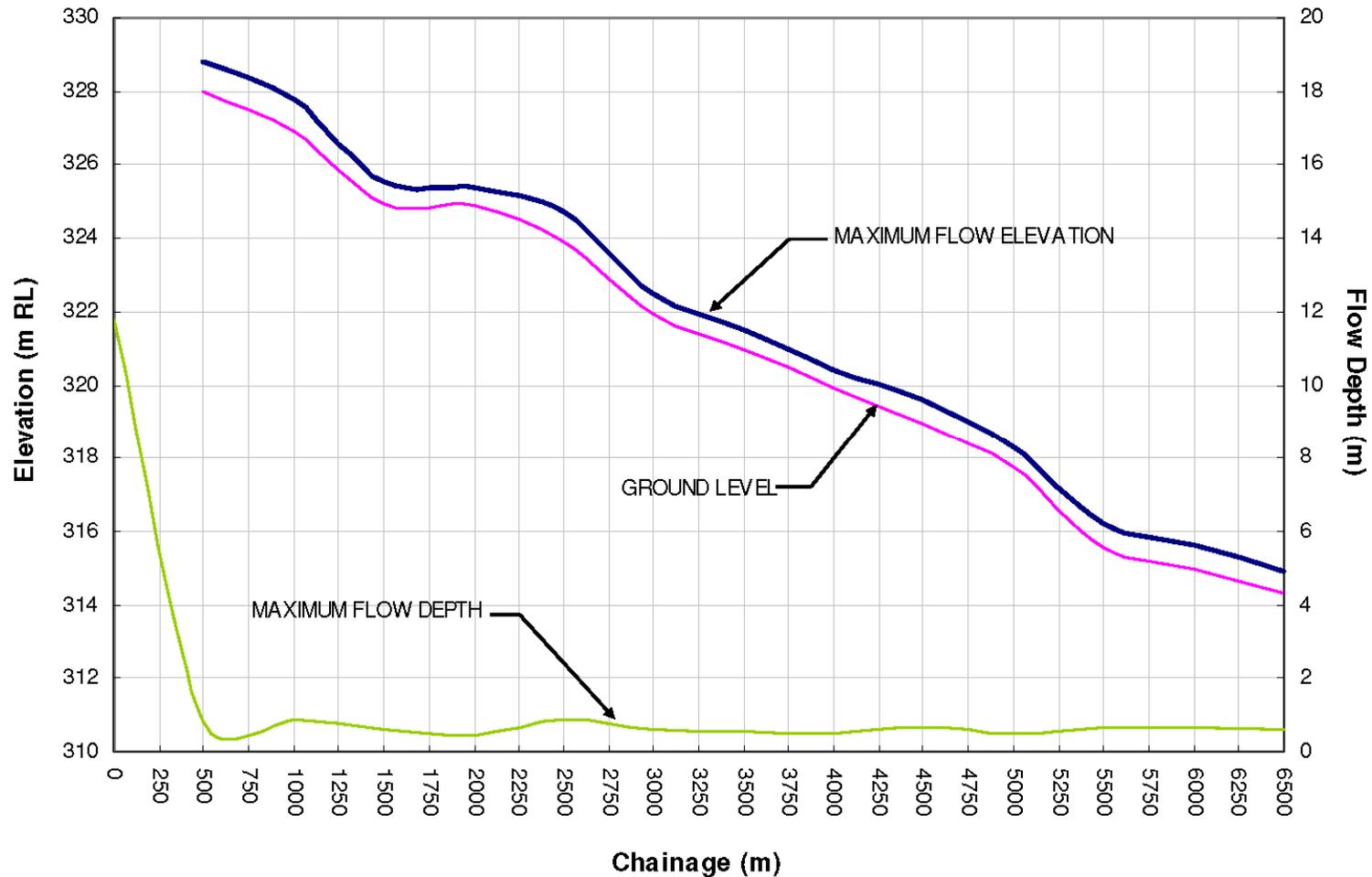
Figure 6 Flow Slide Depth
