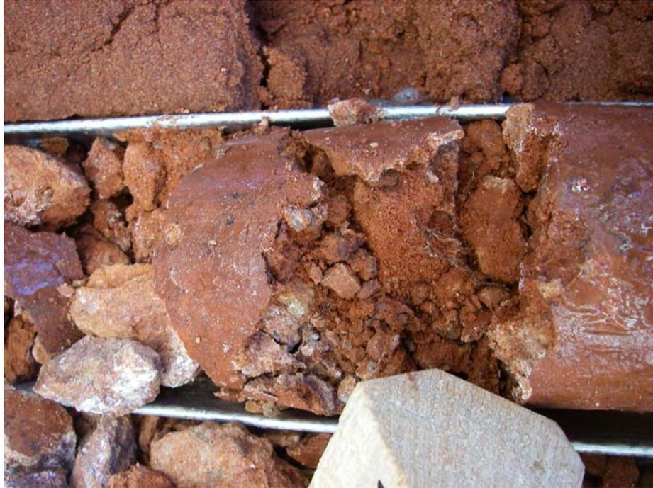
**Figure 11** Interface of Saprolitic Clay and Root Mats Approx. 6 m bgl. This Layer Contains Very Small Voids Created By Roots of Surface Vegetation and Thus Could Potentially be Utilised as Habitat by Troglofauna.
