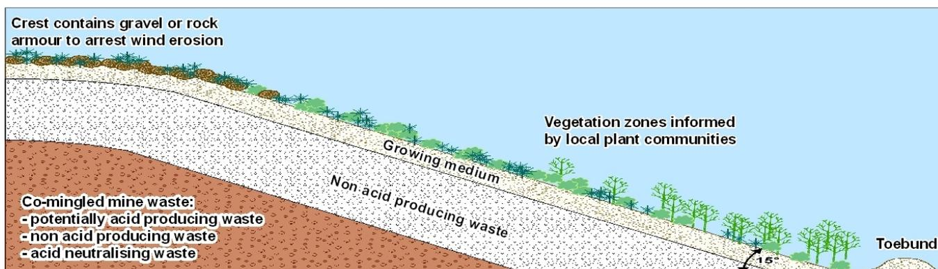
Figure 10.2: Conceptual Waste Landform Cross-section for Tropicana Gold Project
