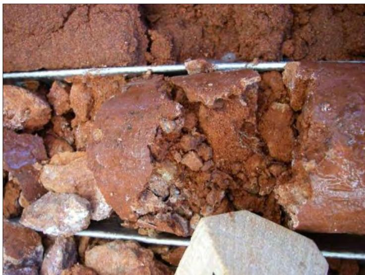
**Plate 6.15: Interface of the Saprolitic Clay and Root Mats approximately 6 mbgl**
