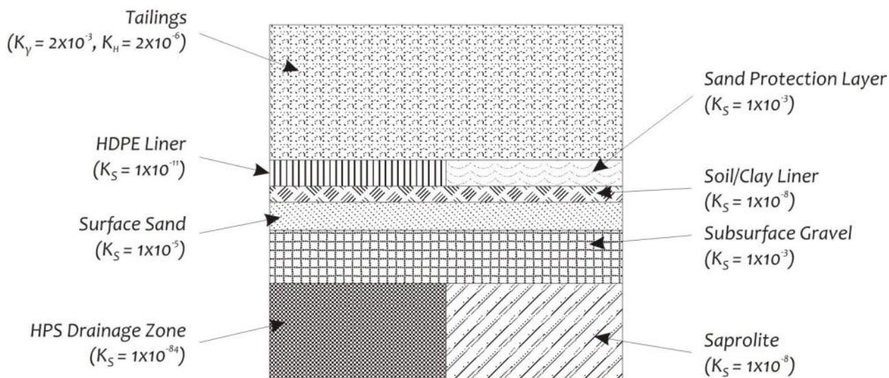
Figure 2.11: Tailings Storage Facility Liner Schematic
