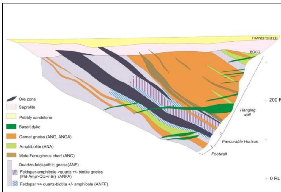
Figure 2.3: Schematic cross section of the Havana Deposit
