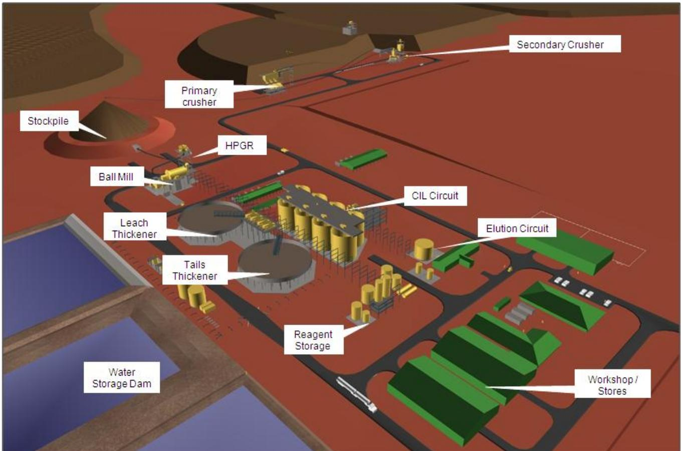
Figure 2.8: Conceptual Processing Plant
