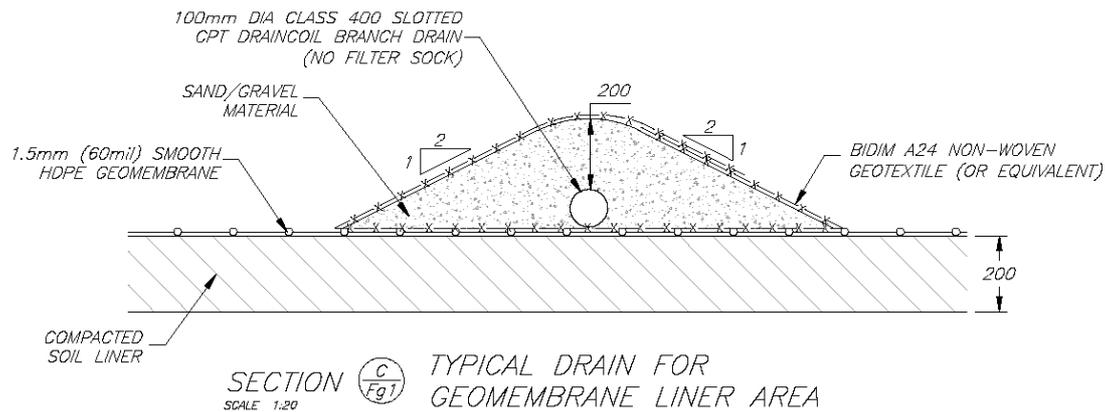
Figure 2.12: Under Drain Configuration over High Density Polyethylene Liner Area
