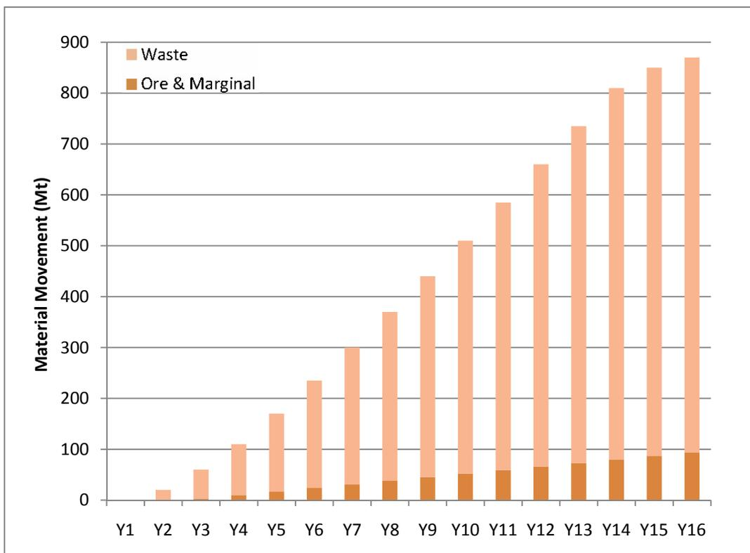
Figure 2.7: Anticipated Accumulative Material Movement
