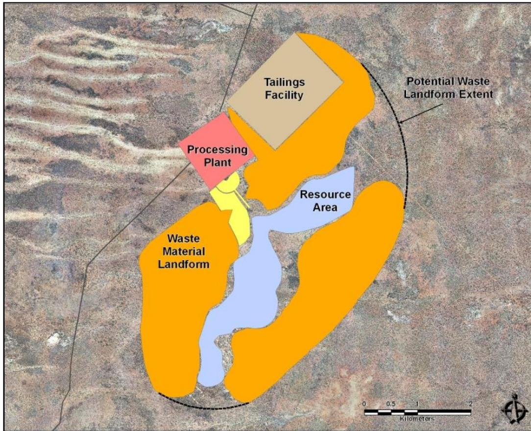
**Figure 2.5: Layout of the Mine and Associated Infrastructure**
